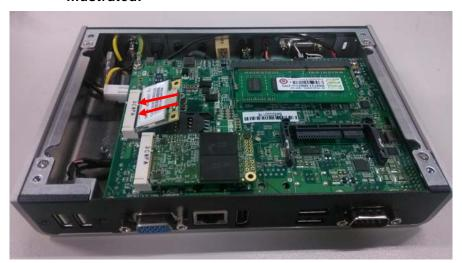
Step 3 Press it firmly down until it is fully located and then fasten the screw per illustrated.
