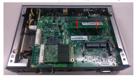
**Step 4** Push the module down, until it is firmly seated by locking two latches on the sides.
