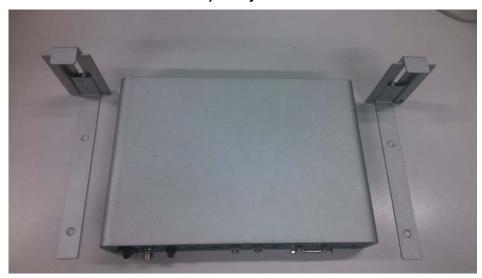
Step 2 Loose the screw of four footpads at the bottom of DSB320-842, and remove footpad.
