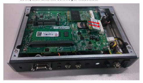
Step 5 Fasten and fix the 3G module with screw per illustrated.
