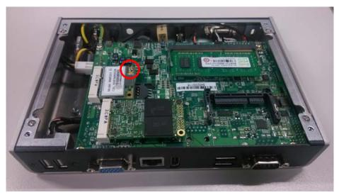
Step 4 Find the Antenna cable and connect it with wireless LAN card.
