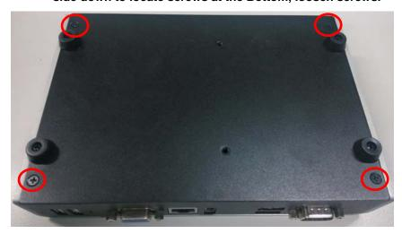
Step 2 Remove the bottom cover and install the Wifi module to the socket per illustrated.
