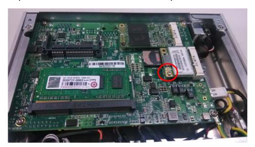
Step 6 Find the Antenna cable and connect it with 3G module.
