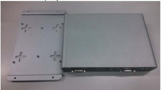
Step 2 After loosing the screw of four footpads at the bottom of DSB320-842, and then put the DSB320-842 under VESA mount kit.
