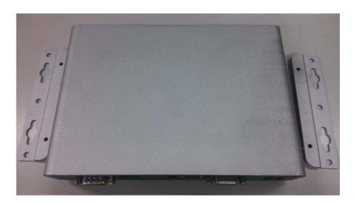
Step 2 Fix the wall mount to the correct location, and fasten all screws.
