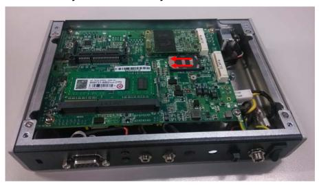
Step 4 Install 3G module. Place the 3G module into the socket and press it firmly down, then affix the screws per illustrated.
