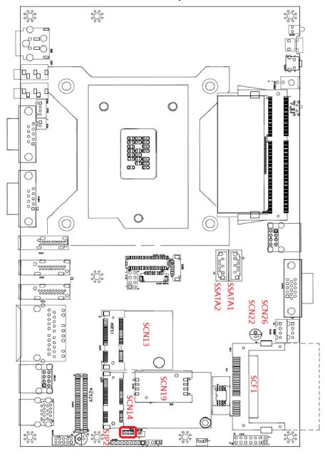
Jumper is a small component consisting of jumper clip and jumper pins. Install jumper clip on 2 jumper pins to close. And remove jumper clip from 2 jumper pins to open. The following illustration shows how to set up jumper.
