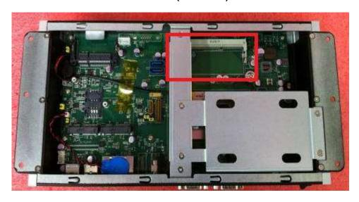
Step 3 Insert the DRAM to the DIMM socket, and then push it down firmly until it is clipped by the socket. Installation completed
