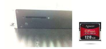
Step 3 Insert the CFast card to the CFast card slot, then finding the CFast cover and screw it.
