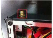
Remove the antenna plug from the top of back cover, and then install the Step 4 antenna on the antenna connector
