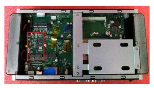
Step 2 Insert the wireless LAN card to the slot. Push it down firmly until it is clipped by the slot.
