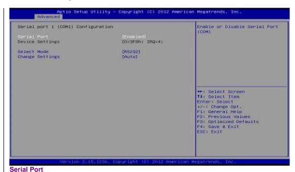
Use this item to enable or disable serial port 1. The optimal setting for base I/O address is 3F8h and for interrupt request line is IRQ4.
