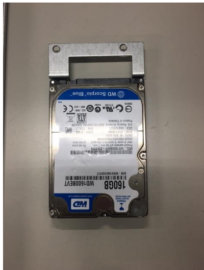
Figure 2-6 Fastening a HDD to the bracket
