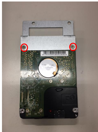
Figure 2-6 Fastening a HDD to the bracket
