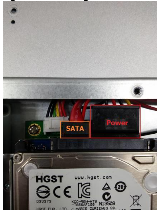
Figure 2-8 Connecting cables to connectors
