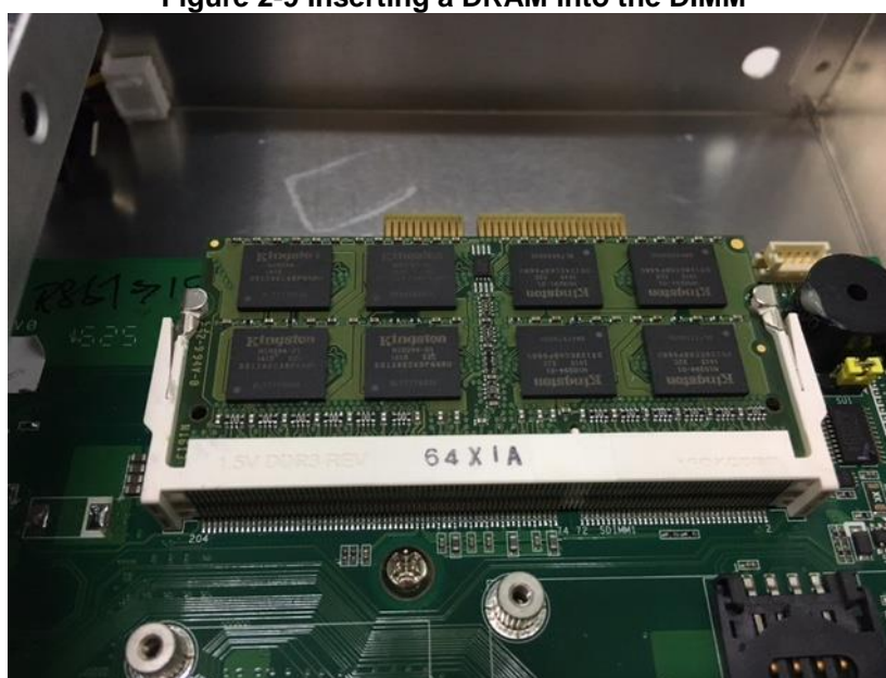
Figure 2-9 Inserting a DRAM into the DIMM
