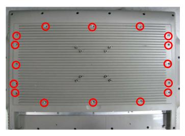
Step 2. Locate and release these screws to open the back cover.
