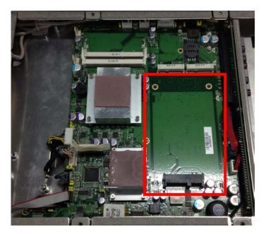
**Step 5.** Fix HDD to the bracket with assembly parts.
