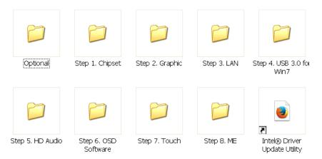
2. Follow the installation sequence arranged from Step 1 to Step 8, as stated in each folder name (see figure above).
