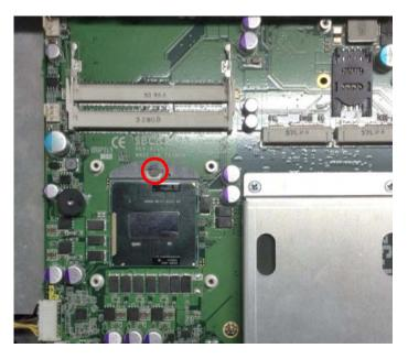
Step 5-3. Place the heat sink on the CPU, and lock it down as marked.
