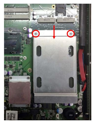
**Step 7.** Close back cover to the chassis, and fasten securely with all screws.
