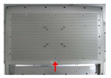
**Step 4.** Release the screw as marked. And remove plates.
