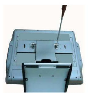
**Step 4.** Then fix the hinge cover with Screw C as marked on figure below.
