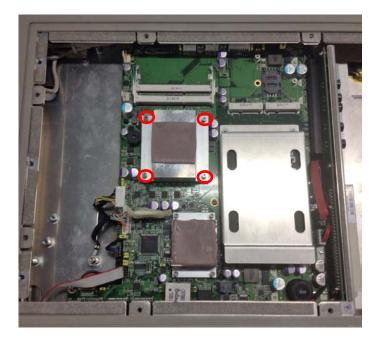
**Step 5-2.** Align pins of the CPU with pin holes of the socket. Be careful of the CPU's orientation, you must align the arrow mark on the CPU with the arrow key on the socket. Place the CPU into the socket, and use a screwdriver to lock it onto the socket as marked.
