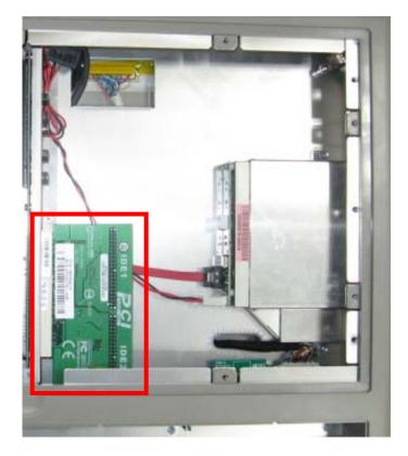
**Step 6.** Fasten with screw as marked.
