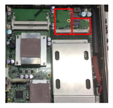
**Step 5.** Insert Mini Card into the socket and push it firmly down until it is fully seated as marked.
