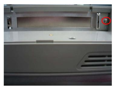
**Step 7.** Close back cover to the chassis, and fasten securely with all screws.
