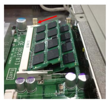
**Step 6-2.** Install the memory module into the socket and push it firmly down until it is fully seated. The socket latches are levered upwards and clipped onto the edges of the SO-DIMM.
