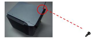
**Step 3** Open the top cover and locate the Hard Disk Drives as red marked.
