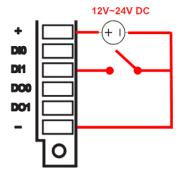
Note: If you are using wet contacts, you must connect COM to power.
