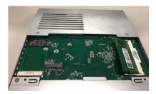
Step 4 The DRAM installation is finished, please fasten all of screws with bracket.
