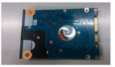
Step 3 Then plug HDD drive in to HDD connector then fasten two screws of the HDD cover bracket
