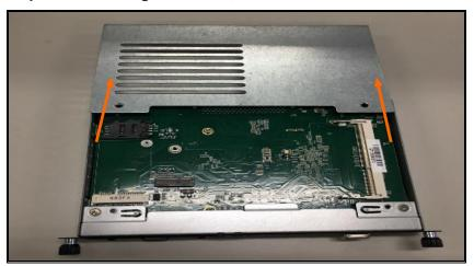
Step 3 Please find the position of Mini PCle & M.2 connectors on the bottom side of OPS.
