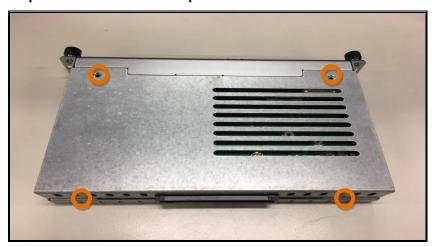
Step 2 After losing the screws, extract the real of chassis out of the module carefully.
