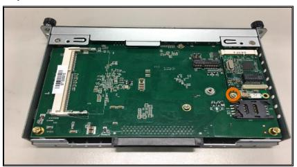
Step 5 Or insert the M.2 module then fasten M4X3 screw carefully.
