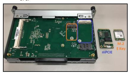
Step 4 Please insert the mPCle module then fasten M2X3 screw carefully.
