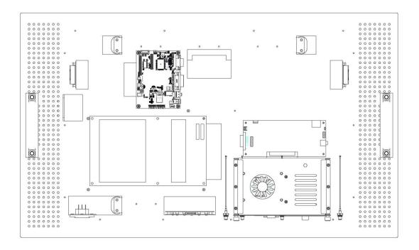
The digital signage OPS300-310 series prototype is based on a OPS compliance display panel with the functional blocks illustrated. It is mainly a 3-board partitioning design consisting of the pluggable module, docking board and the panel control board.
