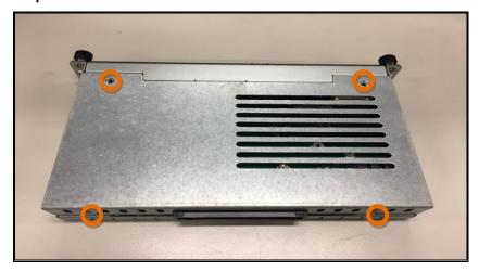
Step 2 After losing the screws, extract the real of chassis out of the module.
