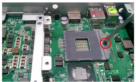
Insert the CPU in to the slot. Please follow the indication on CPU as mark and slot to ensure the proper insertion of the CPU  $\,$
