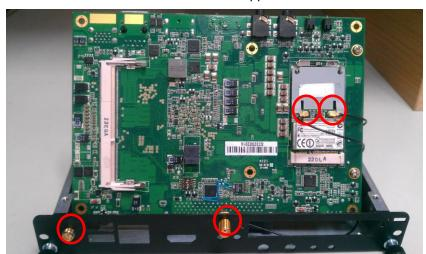
The wireless Module with two antennas application:
