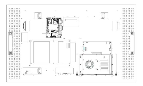
The digital signage OPS871 series prototype is based on a 32" display panel with the functional blocks illustrated. It is mainly a 3-board partitioning design consisting of the pluggable module, docking board and the panel control board.
