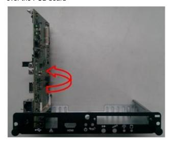
Install Wi-Fi module. Place the Wi-Fi module into the socket and press it firmly down until it is fully located.
