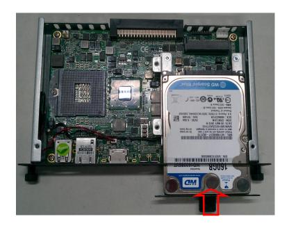
Pull the HDD Mylar to slot-out the HDD drive
