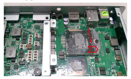
CPU is inserted into the socket and the latch is closed.
