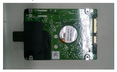
Plug HDD drive in to HDD connector
