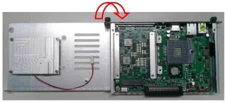
NOTE: Please pull out power cable of system fan while installation
