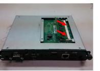
**Step2.3** Align the notch on your DRAM to the key on the socket. Hold the DRAM at a 45-degree angel to the slot and slide it into place. Push the DRAM toward the motherboard until it is snapped firmly into the latch.
