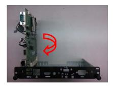
**Step4.2** Loosen the screws of the chassis and PCB board. Turn over the PCB board
