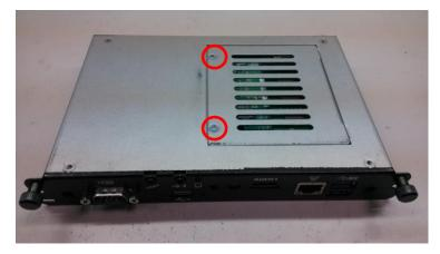
After losing the screws, extract the real of chassis out of the module.
