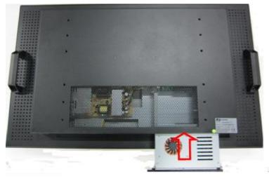
Caution: When plugging OPS880 into an OPS display, make sure the module's heat sink is facing outside of the display. Axiomtek is not responsible for any damage caused by wrong installation.
