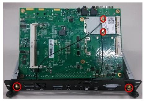
The wireless Module with two antennas application:
