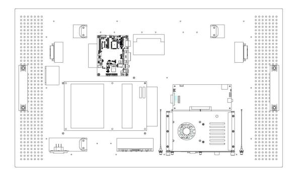
The digital signage OPS880 series prototype is based on a 32" display panel with the functional blocks illustrated. It is mainly a 3-board partitioning design consisting of the pluggable module, docking board and the panel control board.
