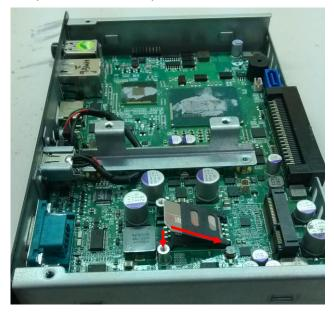
Install 3G module. Place the 3G module into the socket and press it firmly down until it is fully located.
