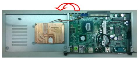
Please loosen the screws of the chassis and PCB board. Turn over the PCB board
