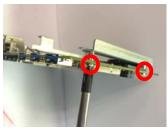
Step 4.2 Affix the HDD bracket to the M/B firmly
