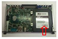
Step 4.4 Plug HDD drive in to HDD connector
