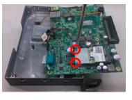
**Step 5.5** Affix the screws per illustrated . Find the Antenna cable and connect 3G card. Screw the antenna connector at expansion I/O side and Install the antenna on 3G card
