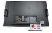
Caution: When plugging OPS885 into an OPS display, make sure the module's heat sink is facing outside of the display. Axiomtek is not responsible for any damage caused by wrong installation
