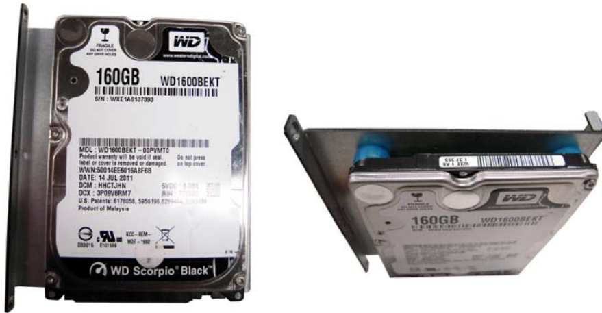
▲ Front and upper views when completed fixing the HDD
