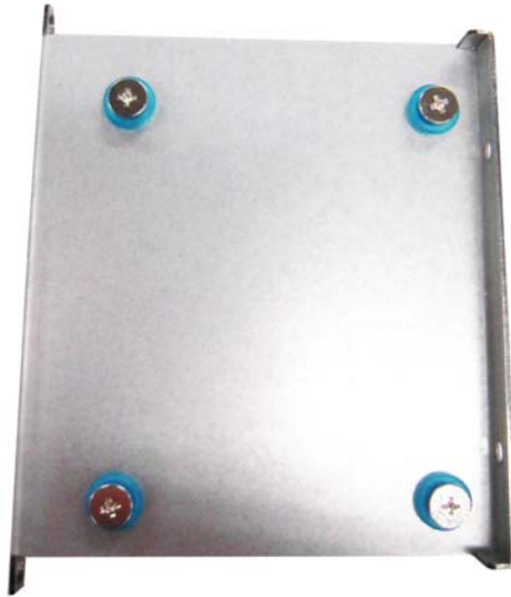
▲ Fix the HDD on the back of bracket
