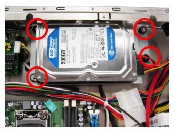
Step 4 Fix the HDD bracket into the main base.
