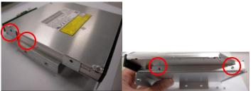
▲ Fixing optical drive by 4 screws.
