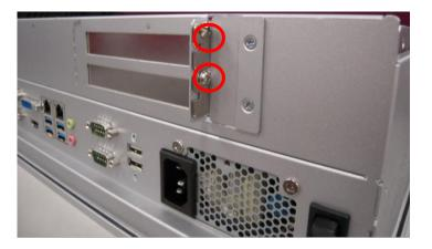
Step 3 Insert the riser card in the socket firmly until it is completely seated. And, insert the add-on card you need to the socket of riser card.
