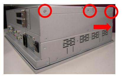
Step 2 Remove the back cover and unscrew 2 screws.
