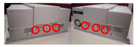
▲ Fixing the bracket by six screws on the left and right side.
