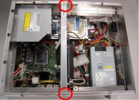
Step 2 Remove the riser card fix kit and plates.
