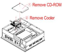
Making sure your CPU settled correctly on the socket. Step 1
