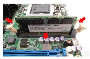
Step 4 The slot latches are levered upwards and latch on to the edges of the SO-DIMM.
