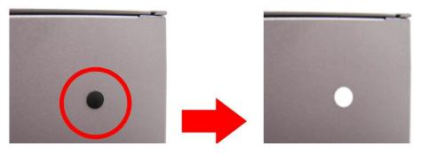
Step 5 Install the antenna on the antenna connector.
