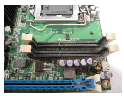
Step 2 Push the latches on each side of the SO-DIMM slot down.
