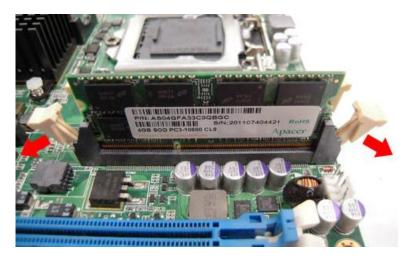
Step 3 Install the SO-DIMM module into the slot and press it firmly down until it seats correctly.
