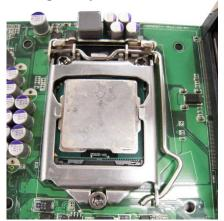
Step 2 Screw the cooling fan supporting base onto the CPU socket on the Motherboard and make sure the CPU fan is plugged to the CPU fan connector. And, Connect the CPU cooler power connector to the FAN1 connector
