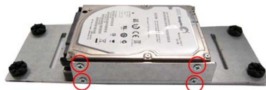
▲ Fix the 2.5" HDD on the right and left side bracket
