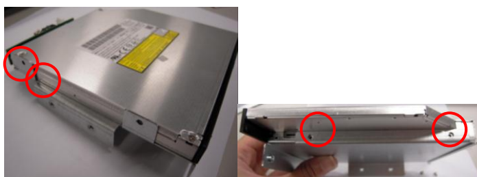
▲ Fixing optical drive by 4 screws.
