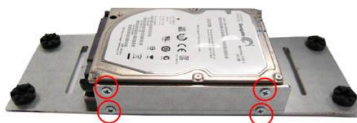
▲ Fix the 2.5" HDD on the right and left side bracket
