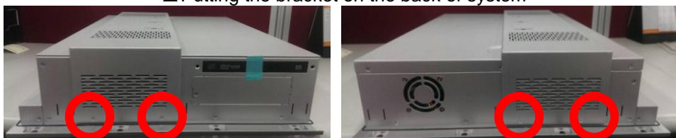
▲ Fixing the bracket by four screws on the left and right side.
