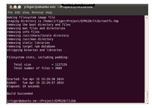
After you have completed a build using LTIB, you will have a target root filesystem in the rootfs directory inside the LTIB install directory.
