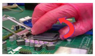
NOTE: Vertical removal is NOT recommended, as it requires higher force and can lead to socket contact damage.
