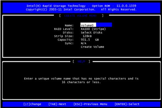
(3)-3-2 When finished, press ENTER to select a RAID level. There are three RAID levels, RAID0, RAID1 and RAID5 & RAID10. Select a RAID level and press ENTER.
