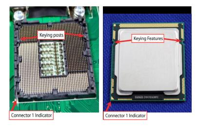
> Grasp the processor with thumb and index finger along the top and bottom edges. (Do not touch the Orientation Notches.) The socket will have cutouts for your fingers to fit into (see image below).
