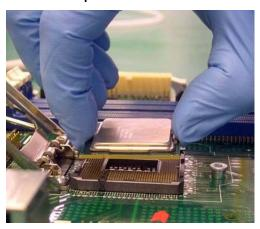
> Verify that package is within the socket body and properly connected to orientation keys.
