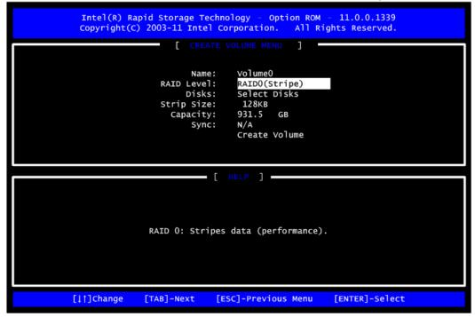
(3)-4 Set the stripe block size. The *KB* is the standard unit of stripe block size. The stripe block size can be 4KB to 128KB. After the setting, press ENTER for the array capacity.
