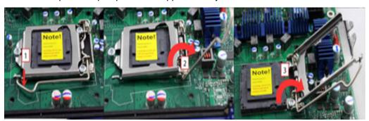
NOTE: Apply pressure to corner with right-hand thumb when opening or closing load lever-otherwise lever will bounce back (as a mouse trap) causing bent contacts.
