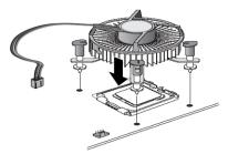
2. Screw the CPU cooling fan onto the board.
