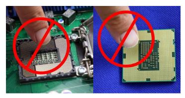
Caution: Never Touch Fragile Socket Contacts to Avoid Damage and Do Not Touch Processor Sensitive Contacts at Any Time During Installation
