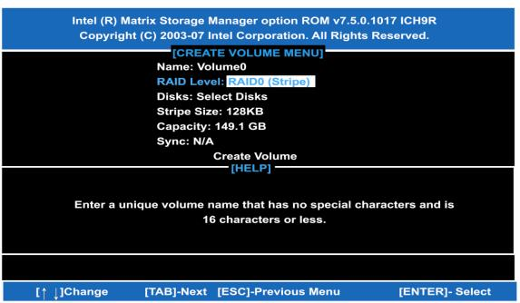
**(3)-4** Set the stripe block size. The *KB* is the standard unit of stripe block size. The stripe block size can be 4KB to 128KB. After the setting, press ENTER for the array capacity.
