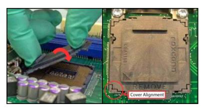
> Close the socket load plate and engage the load lever (see image below).
