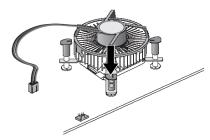
3. Make sure the CPU fan is plugged to the CPU fan connector.
