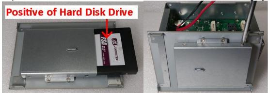
Step 4 Insert the Hard Disk Drive into the bracket and use these screws to fix tightly.
