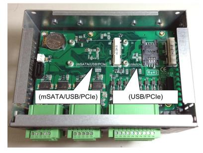
Note: We strongly recommend to choose the wireless socket near heatsink cover side firstly if user only has one wireless inquiry, because the wireless module can be heat dissipated via the thermal parts directly.
