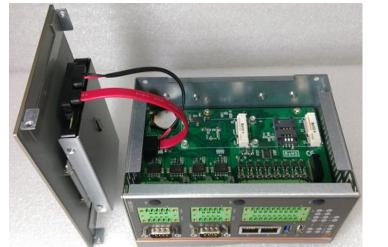
Connecting the SATA+Power HDD cable with Hard Disk Drive. Step 5
