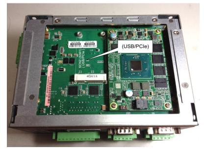
Two wireless sockets are near SSD cover side, one socket supports mSATA/USB/PCIe interface, another supports USB/PCIe interface only.
