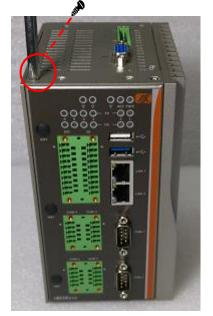
Step 3 Take out the SATA+Power HDD cable & 4pcs of screws for fixing the Hard Disk Drive from the accessory bag.
