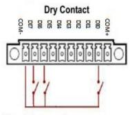
Note: If you are using wet contacts, you must connect COM to power.
