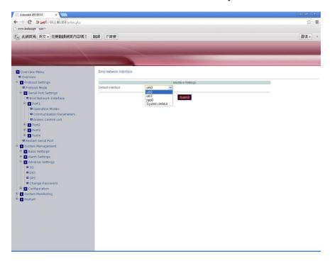
The selection list includes eth0, eth1 and system default. But if 3G dial-up is successful, the ppp0 interface will automatically be added to the list.
