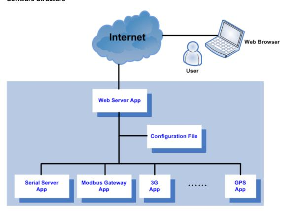
The rBOX610 comes with a set of application software including Serial Server App, Modbus Gateway App, 3G App, GPS App, and Apps for DIO Configuration, SNMP, Alarm, and etc.
