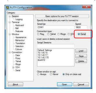
2. Configure the serial port correctly (see image below). Click Open and power on the rBOX630.
