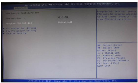
When program PSU setting is [Disabled] 12V or 24V Protection Setting can't modify
