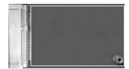
A PCI Express Mini Card can be applied to either PCI Express or USB 2.0. The USB 2.0 support will be helpful during the transition to PCI Express, because peripheral vendors will need time to design their chipsets to have the PCI Express function. During the transition, PCI Express Mini Cards can be quickly implemented by using USB 2.0.
