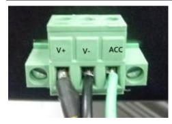
ACC means "accessories". Mainly, it acts both notice signal to all electronical devices, and also provides DC from battery.
