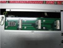
one slot contains an internal SIM card slot which can support 2G/3G/4G modules.
