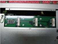
one slot contains an internal SIM card slot which can support 2G/3G/4G modules.
