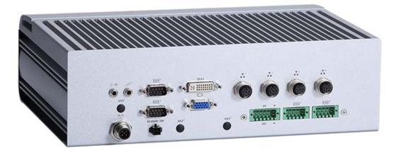
Pin + is connected to voltages between 9 and 36V
